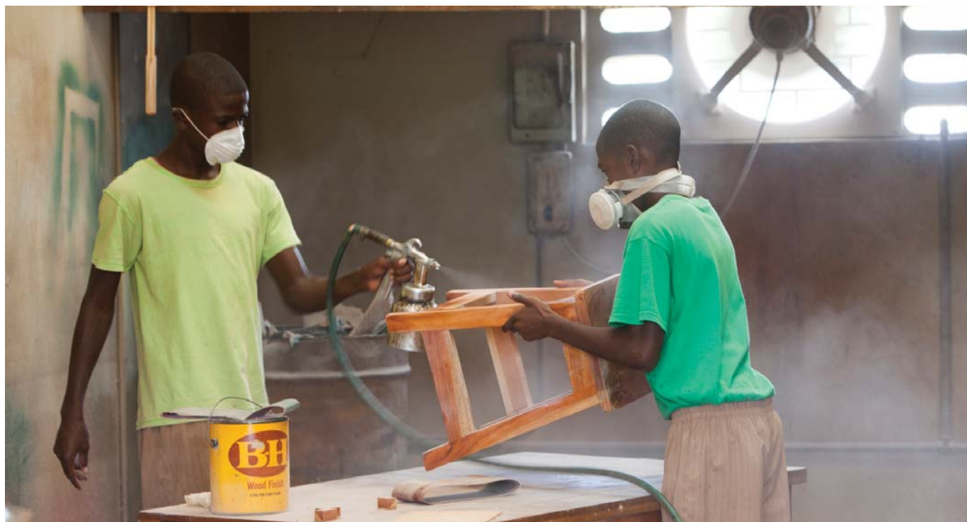
Woodwork students applying varnish to one of the stools made for the institution - Alpha, Jamaica.
